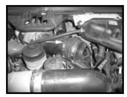
Step 11 Install the flex boot onto the turbo inlet.
