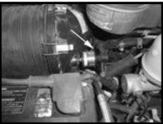
Step 3 Remove the filter minder from the back of the airbox.
