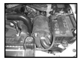
Step 5 Remove the factory air box from the vehicle by lifting up and out on the backside of the airbox.
