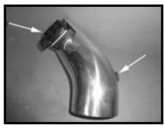
Step 8 Using the supplied screws, install the MAFS onto the tube. Install the grommet into the tube as shown.
