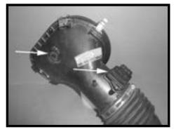
Step 7 Remove the MAFS from the factory intake tube. Remove the factory grommet for the filter minder.
