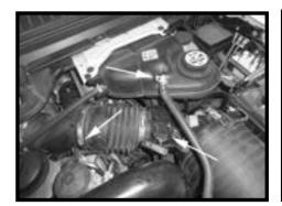
Step 2 Disconnect the electrical connector at the Mass Air Flow Sensor (MAFS). Disconnect the radiator overflow line and loosen the clamp at the end of flex inlet.
